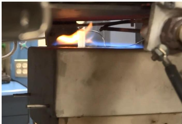
Samples subject to heat flux exposure of 50Kw/m<sup>2</sup>
