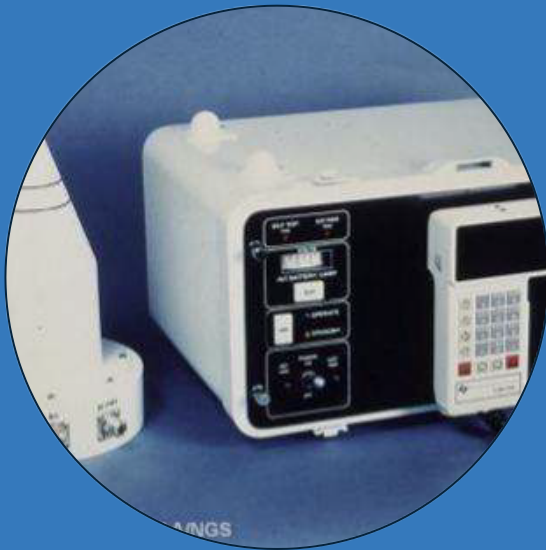
1st commercial GPS receiver in 1981 Weight: 53 lbs; Cost: $119,900
