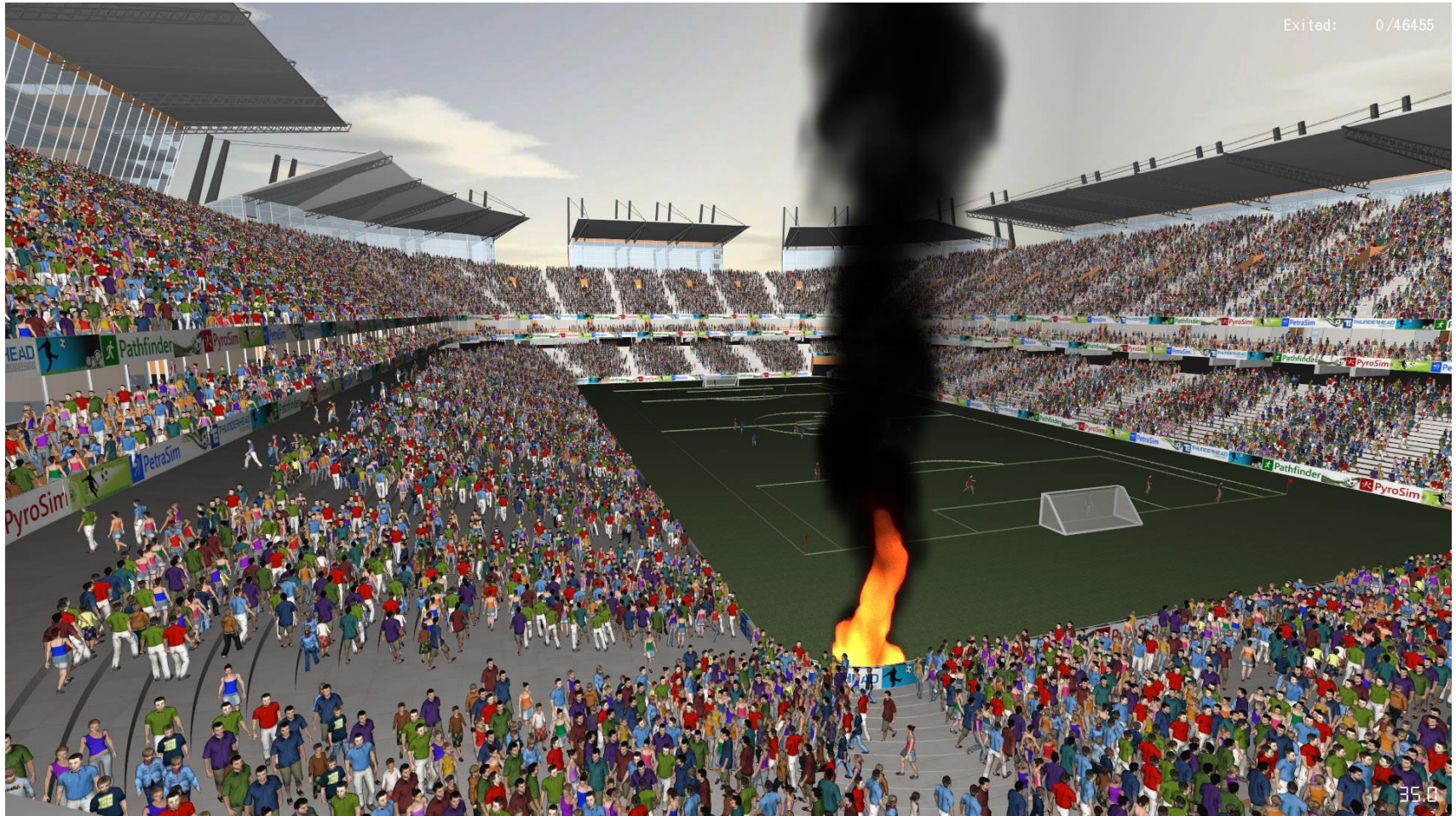
Evacuation / CFD Model Visualisation (Courtesy of Thunderhead Engineering)
