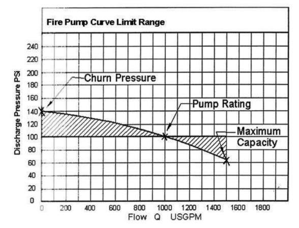
NFPA 20 recommends that pumps should run at 90% - 140% of rated capacity
