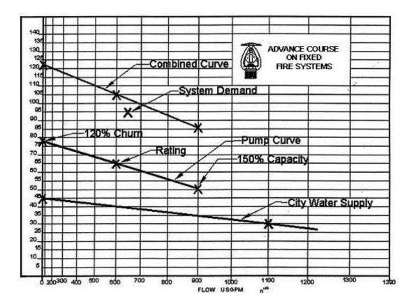
System demand point falls below the combined curve which means pump is adequate
