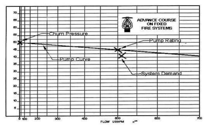
System demand point is below pump curve; pump will satisfy demand. Demand point is 3 PSI below pump curve; the next pump rated at 500 GPM @ 50 PSI, is a better choice.
