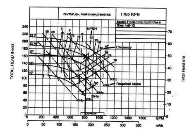
800 GPM at 160 feet of discharge head is required
