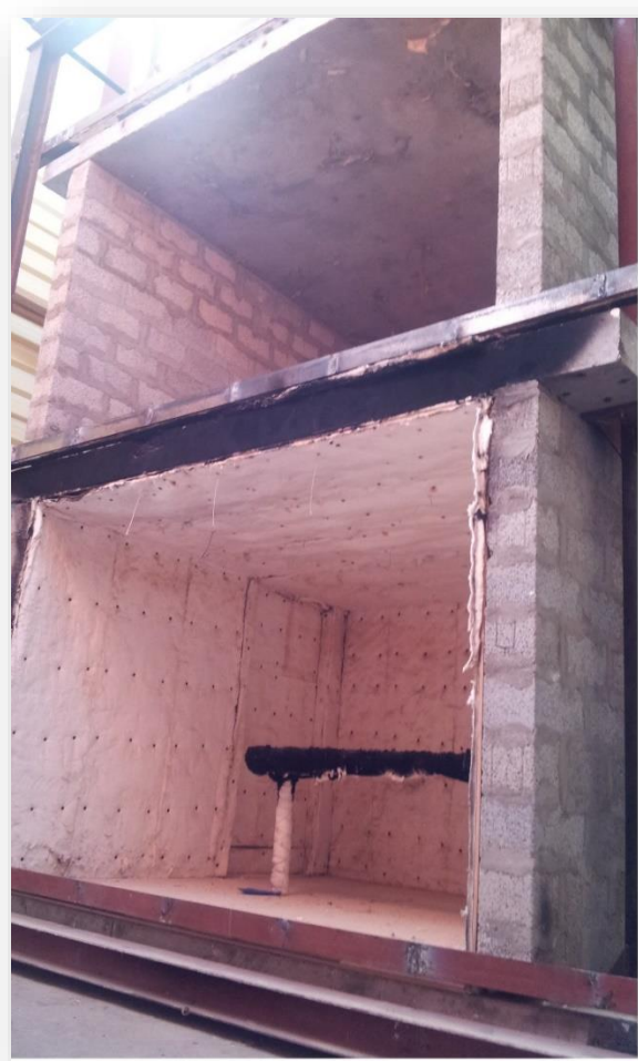
Intermediate Scale Multi-storey Test Apparatus or ISMA, used to conduct the NFPA 285 for Cladding Systems test and the ASTM E2307 test Firestops
